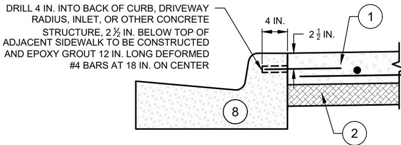
**CONSTRUCTION JOINT OF SIDEWALK ADJACENT TO BACK OF CURB, DRIVEWAY RADIUS, INLET, OR OTHER CONCRETE STRUCTURE**
