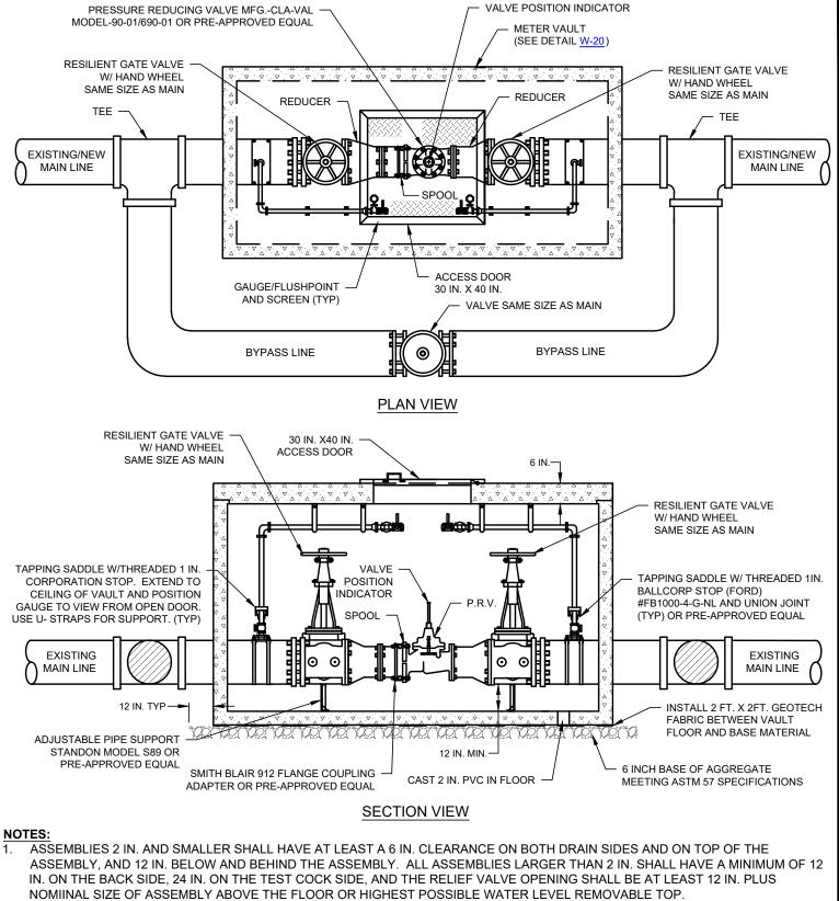
THE ASSEMBLY SHALL BE READILY ACCESSIBLE FOR TESTING AND MAINTENANCE, WITH A MINIMUM CLEARANCE OF 12 IN. ALL AROUND THE ASSEMBLY.
