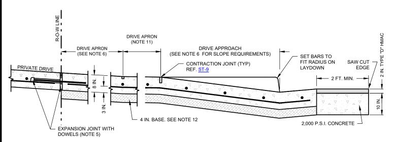
SECTION A - NEW APPROACH ON EXISTING ASPHALT STREET (NO SCALE)
