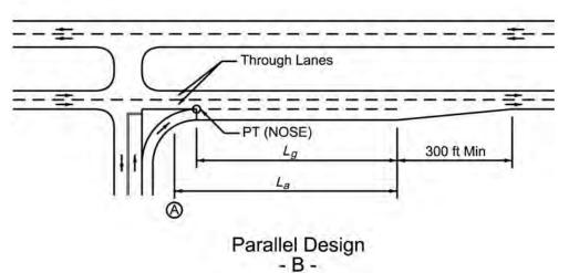
Figure 3-14. Examples of Tapered and Parallel Acceleration Lanes.
