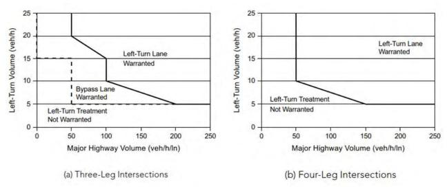
Figure 3-8. Suggested Left-Turn Warrants Based on Results from Benefit-Cost Evaluations for Intersections on Two-Lane Highways in Rural Areas.
