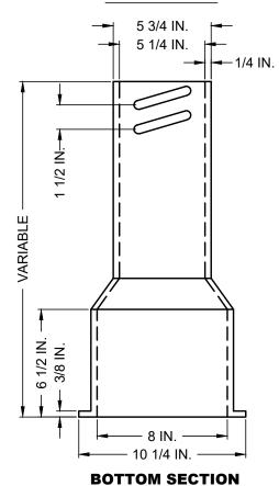
TYLER/UNION 6850 SERIES 462-S OR 562-S CAST IRON TWO-PIECE VALVE BOX OR PRE-APPROVED EQUAL.
