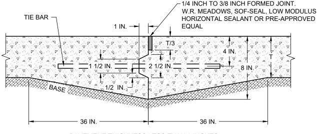
PAVEMENT THICKNESS LESS THAN 8 INCHES
