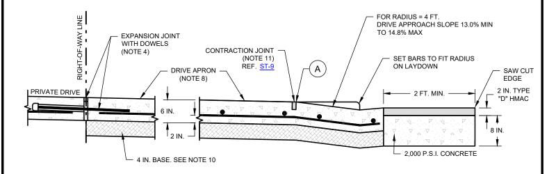
(A) ELEVATION 1 IN. MIN. TO 2 IN. MAX ABOVE TOP OF "ADJACENT CURB FOR RADIUS = 4 FT.
