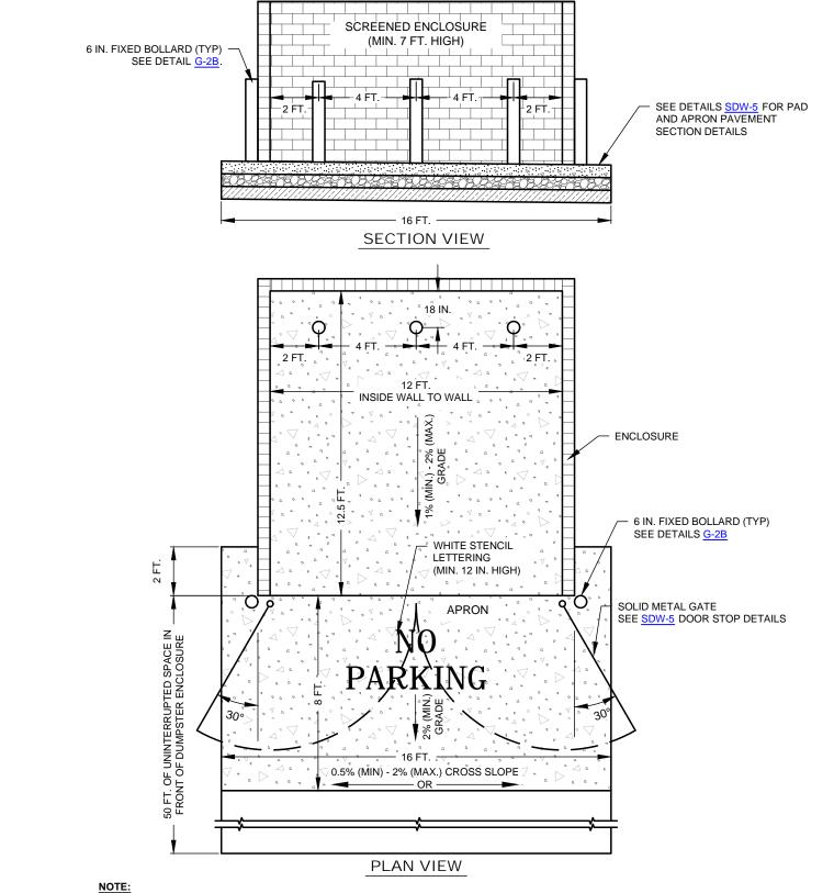
APRON SHALL BE GRADED TO DRAIN TOWARDS APPROVED DRAINAGE PATH WITH A MINIMUM 2% LONGITUDINAL SLOPE AND A MINIMUM 0.5% CROSS SLOPE AND MAXIMUM 2% CROSS SLOPE. ANY DESIGNS THAT PROPOSE TO EXCEED 2% CROSS SLOPE SHALL REQUIRE THE APPROVAL OF THE DIRECTOR OF SOLID WASTE DEPARTMENT.
