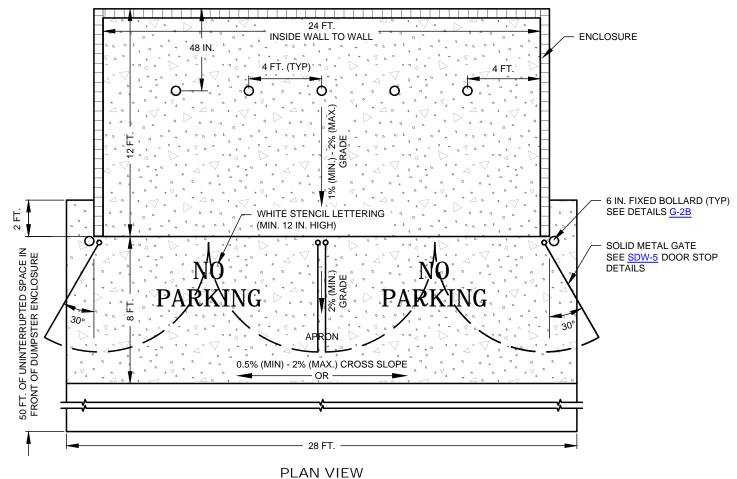
APRON SHALL BE GRADED TO DRAIN TOWARDS APPROVED DRAINAGE PATH WITH A MINIMUM 2% LONGITUDINAL SLOPE AND A MINIMUM 0.5% CROSS SLOPE AND MAXIMUM 2% CROSS SLOPE. ANY DESIGNS THAT PROPOSE TO EXCEED 2%  $^{\circ}$ CROSS SLOPE SHALL REQUIRE THE APPROVAL OF THE DIRECTOR OF SOLID WASTE DEPARTMENT.
