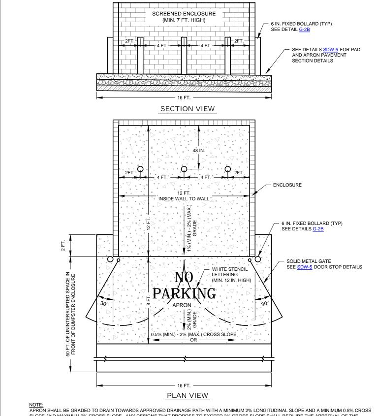
APRON SHALL BE GRADED TO DRAIN TOWARDS APPROVED DRAINAGE PATH WITH A MINIMUM 2% LONGITUDINAL SLOPE AND A MINIMUM 0.5% CROSS SLOPE AND MAXIMUM 2% CROSS SLOPE. ANY DESIGNS THAT PROPOSE TO EXCEED 2% CROSS SLOPE SHALL REQUIRE THE APPROVAL OF THE DIRECTOR OF SOLID WASTE DEPARTMENT.
