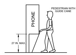
PROTRUDING OBJECTS OF A HEIGHT  $\leq$  27 IN. ARE DETECTABLE BY CANE AND DO NOT REQUIRE ADDITIONAL TREATMENT.
