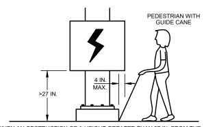
WHEN AN OBSTRUCTION OF A HEIGHT GREATER THAN 27 IN. FROM THE SURFACE WOULD CREATE A PROTRUSION OF MORE THAN 4 IN. INTO THE PEDESTRIAN CIRCULATION AREA, CONSTRUCT ADDITIONAL CURB OR FOUNDATION AT THE BOTTOM TO PROVIDE A MAXIMUM 4 IN. OVERHANG.
