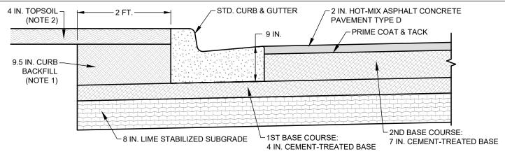
$CC3 \text{ (F)} \quad \begin{array}{ll} \text{TYPICAL FLEXIBLE PAVEMENT SECTION:} \\ \text{COMMERCIAL COLLECTOR STREET ( P.I. } \geq 40) \end{array}$
