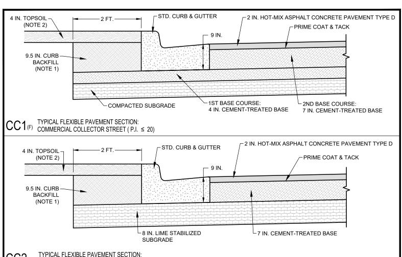
CC2(F) TYPICAL FLEXIBLE PAVEMENT SECTION: COMMERCIAL COLLECTOR STREET (20 < P.I. < 40)
