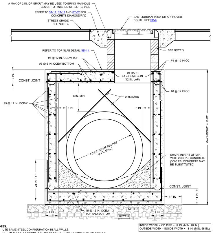
SET MANHOLE AT CORNER NEAREST OUTLET PIPE BEARING ON TWO WALLS.
