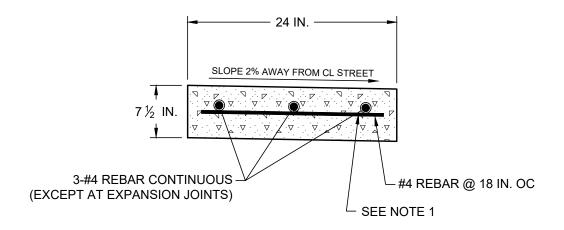
1. TRANSVERSE BARS MAY BE OMITTED WHEN CONCRETE FOR RIBBON CURB IS PLACED WITH A SELF-PROPELLED CURB MACHINE THAT PROVIDES CORRECT PLACEMENT OF THE LONGITUDINAL BARS
