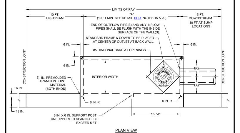
INTERIOR WIDTH = OUTSIDE DIAMETER OF LARGEST PIPE + 12 IN., 36 IN. MINIMUM
