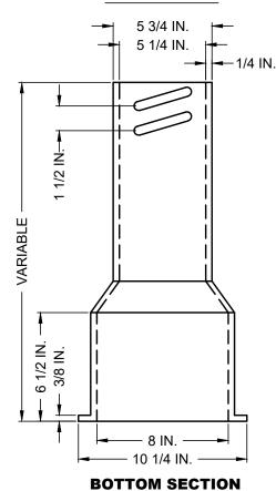
TYLER/UNION 6850 SERIES 462-S OR 562-S CAST IRON TWO-PIECE VALVE BOX OR PRE-APPROVED EQUAL.
