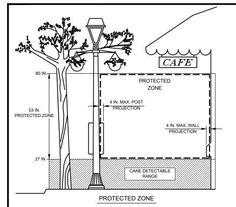
NOTE: IN PEDESTRIAN CIRCULATION AREA, MAXIMUM 4 IN. PROJECTION FOR POST OR WALL MOUNTED OBJECTS BETWEEN 27 IN. AND 80 IN. ABOVE THE SURFACE.
