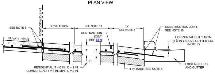
SECTION A - NEW APPROACH ON EXISTING STANDARD CURB AND GUTTER
