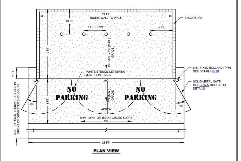
APRON SHALL BE GRADED TO DRAIN TOWARDS APPROVED DRAINAGE PATH WITH A MINIMUM 2% LONGITUDINAL SLOPE AND A MINIMUM 0.5% CROSS SLOPE AND MAXIMUM 2% CROSS SLOPE. ANY DESIGNS THAT PROPOSE TO EXCEED 2%CROSS SLOPE SHALL REQUIRE THE APPROVAL OF THE DIRECTOR OF SOLID WASTE DEPARTMENT.
