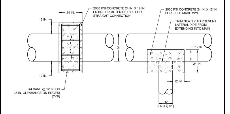
**NOTE:** CONCRETE TO BE PLACED COMPLETELY AROUND PIPE.
