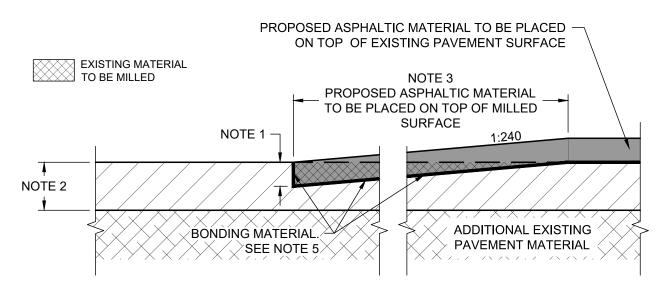
TRANSITION TO AND FROM PLACEMENT OF ASPHALTIC MATERIAL ON EXISTING PAVEMENT SURFACE
