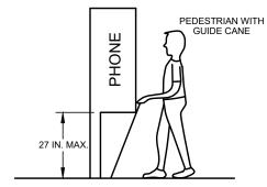
PROTRUDING OBJECTS OF A HEIGHT  $\leq$  27 IN. ARE DETECTABLE BY CANE AND DO NOT REQUIRE ADDITIONAL TREATMENT.
