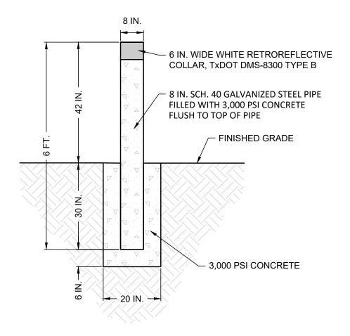
1. BOLLARDS PLACED IN SERIES TO BE SPACED MAXIMUM 5 FT. APART MEASURED FROM BOLLARD CENTER TO CENTER UNLESS OTHERWISE SHOWN IN PLANS
