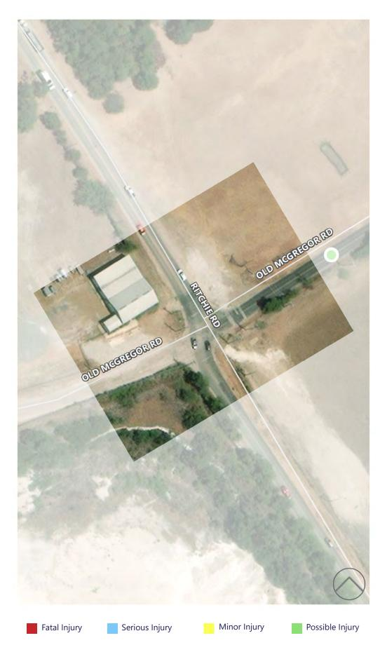
The intersection of Ritchie Road and Old McGregor Road is an all way stop controlled skewed-intersection. The speed limit approaching this intersection is 30 mph. Currently the intersection has an off-set geometry posing a safety challenge for drivers. Non-injury collisions have been reported at this intersection.
