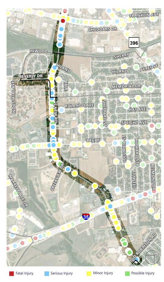
S New Road, a four-lane major arterial with a center two-way left turn lane, provides access through commercial and residential areas from Franklin Avenue to Old Robinson Road. The speed limit is set at 45 mph along the corridor. This corridor provides access to University High School and the Waco ISD Stadium.
