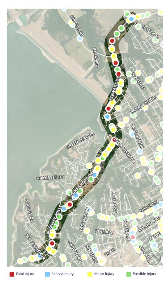
Lake Shore Drive, a four-lane minor arterial with a center two-way left turn lane, runs through a mix of commercial and residential areas from Mt Carmel Drive to N 19th Street. The speed limits vary, set at 40 mph from Mt Carmel Drive and Hillcrest Drive and 50 mph between Hillcrest Drive and N 19th Street. Lakeshore Drive is within 0.25 mile of Vanguard Preparatory School.
