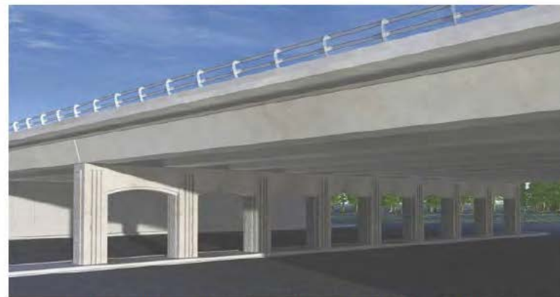
Multiple Column Bent – matches the “Art Deco” look of the Brazos River (BRG)
